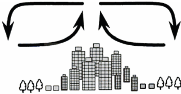
Figure 14.15. Generalized urban heat island atmospheric circulation.
